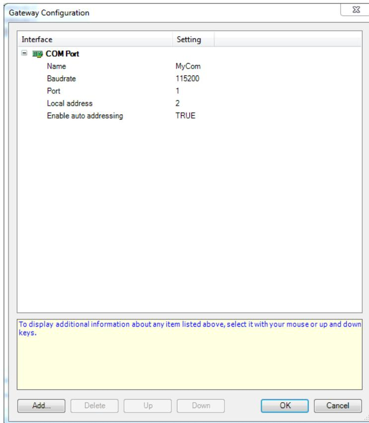
If any of the configuration settings are missing click "Add..." and select "Add configuration setting..". Make sure to restart the gateway after changing configuration. This can be done by right clicking on the gateway in the system tray and selecting "Stop Gateway" followed by "Start Gateway".
